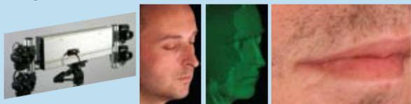
Dolphin's new Di3D High Definition Facial Camera System lets you accurately capture three-dimensional surface contours of any patient's face in high resolution. Using Dolphin 3D, this facial data seamlessly integrates with the patient CBCT data to create a complete virtual patient model. The image can be easily analyzed and manipulated.
